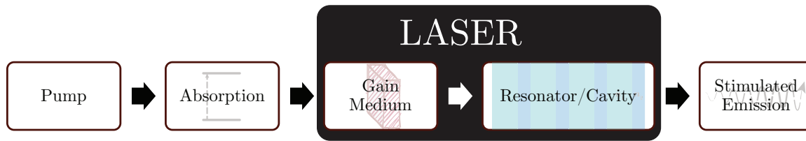
Figure 1.1: A simplified depiction of a laser system.
